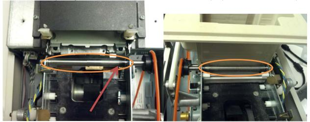
Notice in picture above left side of roller is clean and right side is black. Clean roller until it is completely clear. (no black).
