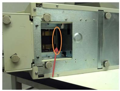
After cleaning the top two rollers turn loader on its side while the rollers are still spinning and clean the bottom two rollers. 4 Rollers total.
