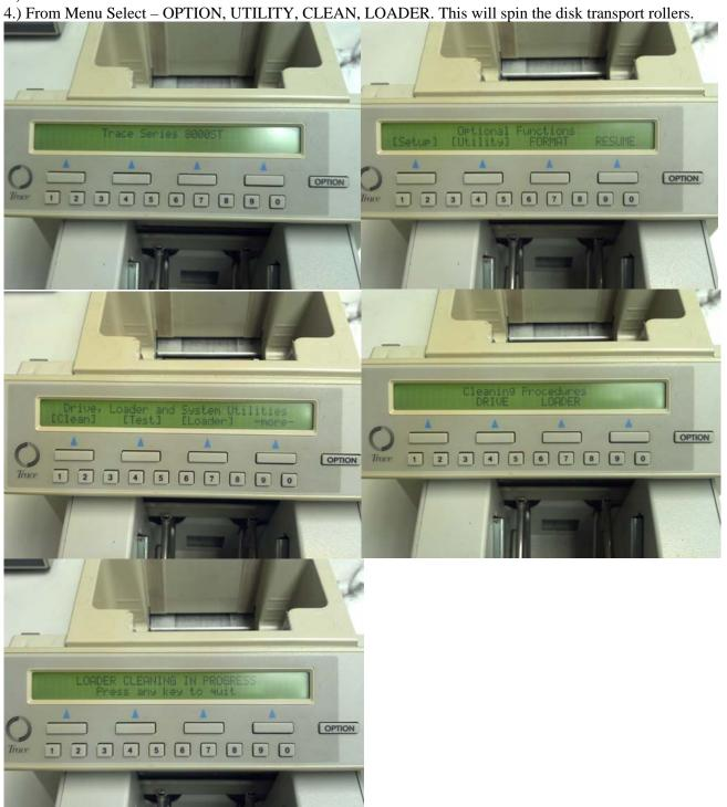
While rollers are spinning, use hand towel wet with IPA or Windex and put pressure on roller while spinning
