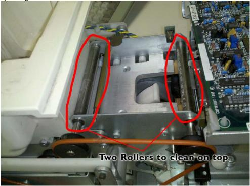
This will clean the roller. Repeat this process for all 4 rollers. Turn loader on side to access 2 bottom rollers.
