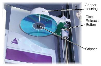
7. Manually move the gripper down to the top of the carousel as shown.
