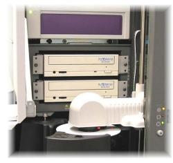
8. If the carousel is not centered between the four points as shown, adjustment is required.
