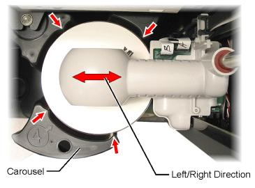
9. To move the gripper hub left or right, remove the disc and loosen the T15 screw located under the gripper housing as shown.
