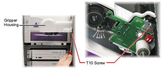
12. Grasp the top of the griper housing and move the housing until the disc is centered between the carousel points.
