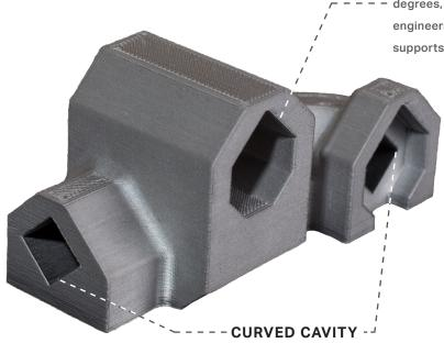
A curved, diamond-shaped cavity houses the series of ball bearings that transmit force.
