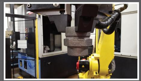
Dixon Valve primarily produces valves and fittings, these grippers also require strength and chemical resistance, as well as wear resistance from repeated use. "To that end, we utilise the Markforged parts as our transfer gripping system," adds de Arriz.
