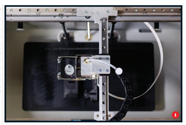
e've covered the Markforged nylon and carbon fibre machine, the Mark Two, extensively in the last few months (see both the January and February issues). The ability to mix a nylon-based material with single strand fibres (including carbon, glass and Kevlar) certainly impressed us.
