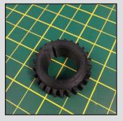
Test part: Timing case pinion
