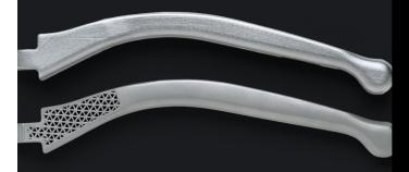
ADAM enables the creation of unique geometries such as closed-cell honeycomb infill. Parts can be printed like the structure of bones - a closed cell inner core encased in a solid outer shell. This geometry is not possible using traditional subtractive manufacturing processes
