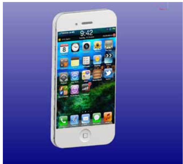
Fig. 2 ColourIT applies color to the 3D digital files prior to slicing in SliceIT.
