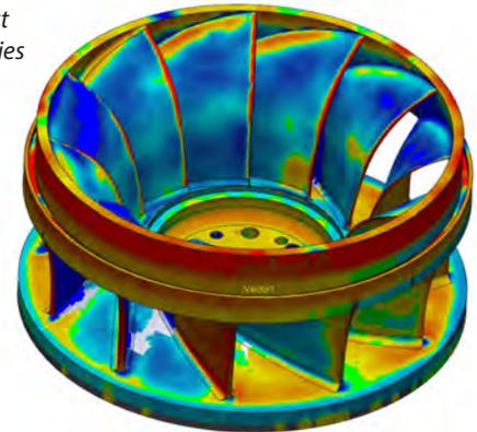
Other factors impacting 3D print accuracy include part size and geometry. Some 3D printers provide varying levels of print preparation tools for fine tuning accuracy for specific geometries. Accuracy claims by manufacturers are usually for specific measurement test parts and actual results will vary depending on part geometry, so it is important to define your application accuracy requirements and test the 3D printer under consideration using your specific application geometry.
