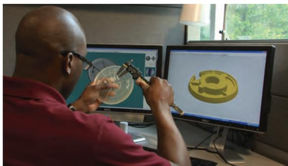
*Holding and measuring a printed part offers a better understanding than viewing a rendering on screen*
